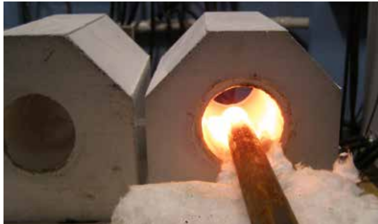
Heating a 75 mm diameter bar to 1100 °C (2012 °F) for hot heading. An eight-position coil was used to provide one hot bar end every 20 seconds to the robot for loading into the press.
